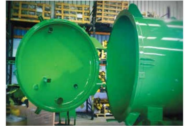
**Fully Opening Rear Door:** These doors are mounted on hinges. They are locked by six threaded hooks.
