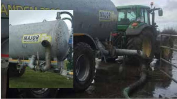
**Autofiller:** 6" or 8" hydraulic coupler. It is ideal for slurry pits that are difficult to access. It reduces your filling time by half. A galvanised tripod is supplied as standard.
