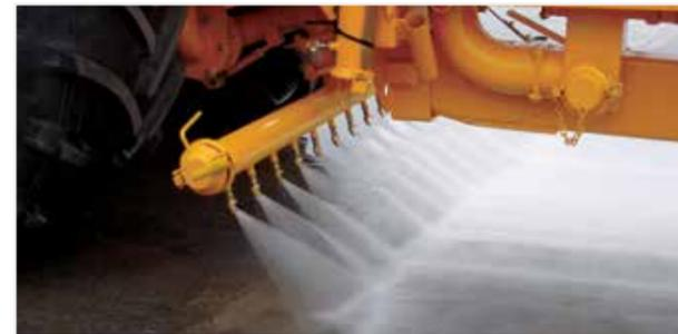
**Road Blaster Unit:** This unit is fitted beneath the tanker for high-pressure road washing. The angle of the nozzles can be adjusted for tough conditions
