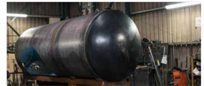
The joints on the tank are welded to ensure a high-quality and visually perfect weld seam.
