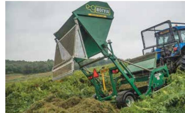
The MAJOR MJ2000 Flail Collector is designed to perform even in the most extreme conditions and is suitable for use with larger compact and agricultural type tractors.
