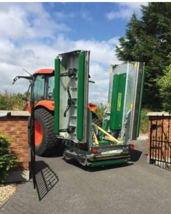
wings folded, there's an LED road lighting kit available, and a transport width of 1.9m makes it straightforward to gain entrance where tight access is an issue. You also have peace of mind with a 3-year MAJOR warranty on your mower. The 1.9m transport width allows for easy access with wing lock for safe road transportation
