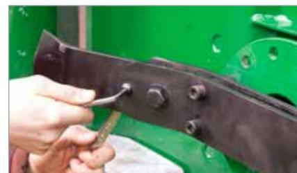
Two in one blade system, rigid and swinging
