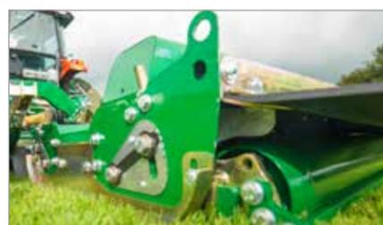
Cutting height adjustment system from 10 - 110mm
