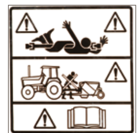
PTO entanglement hazard - keep clear of PTO drives.
