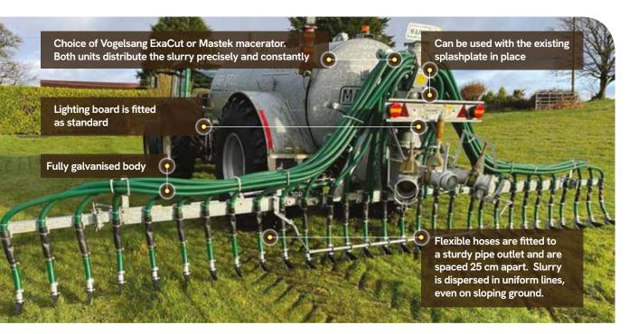
Each unit is divided into three sections. The middle section behind the tanker is lifted by a lateral pipe connected to each wing. When the wings are folded into transport position, the midsection also lifts. This protects the unit when reversing and for safe road transport.
