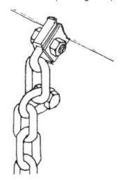
To prolong the life and maintain the efficiency of the rotor (Flail tube), the flail chains must balance. Any work carried out on one chain must be repeated on the flail chain opposite the rotor to maintain the equilibrium of the rotor. Premature flailing of the bearings can result if the rotor is used for long periods in an out of balance state.
