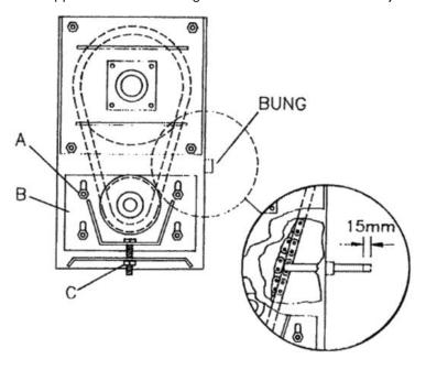
4. With continual use it is possible that the flail chain could stretch until the flail heads hit the side of the drum. To prevent this happening, shorten the flail chain by inserting a M10 x 25 bolt and self-locking nut, through a chain by approx. 18mm. an alternative method is to remove two links. (See Figure 4)
