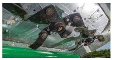
The three-rotor blade system with a 150mm (6") overlap, gives precise and even cutting. High blade tip speeds combined with four blades per rotor delivers intense shredding of material with no clumping. From heavy grass swards and uneven terrain to wet and dry lawns, the Synergy deck handles various conditions with ease.
