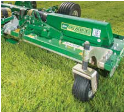
Option of a castor wheel per wing for racecourse applications
