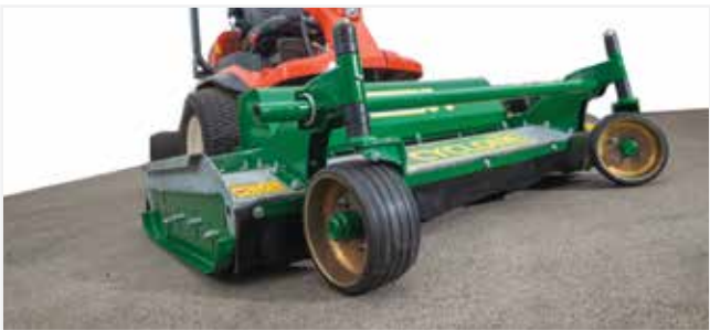
Cutting height adjustment system from 10 - 110mm
