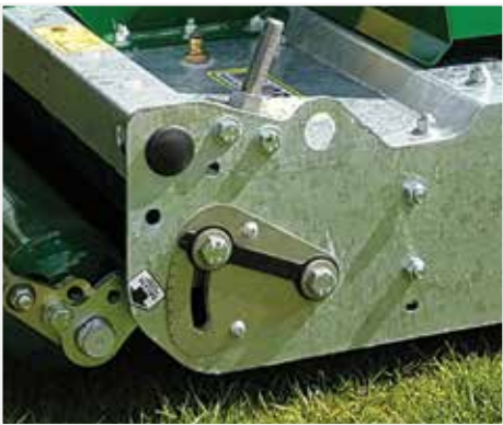
10-130mm height adjustment for year round mowing
