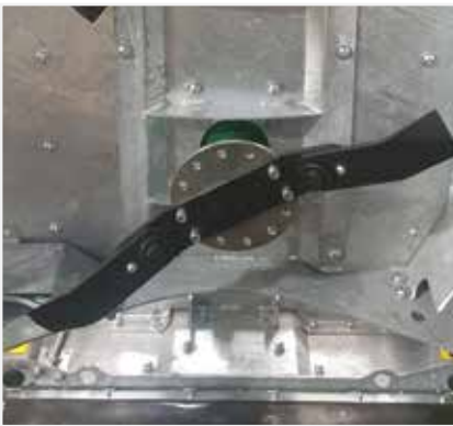
Two in one blade system, rigid and swinging
