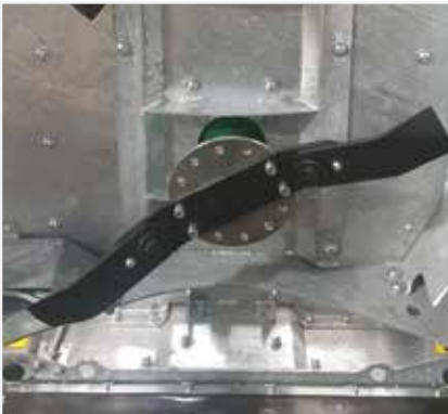
Two in one blade system, rigid and swinging
