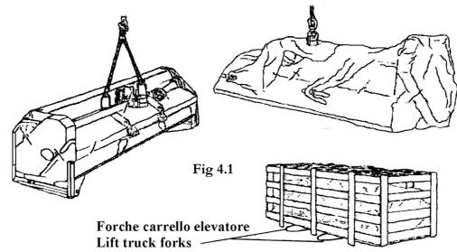
Use a lift truck, a crane or other equipment with an adequate carrying capacity to lift the implement, checking its weight in the table. Check that the load is stable and well positioned on the truck forks or crane hook. Keep the load as low as possible when moving the implement. This will ensure greater stability and visibility. Set the forks to their maximum width if a lift truck is used.
