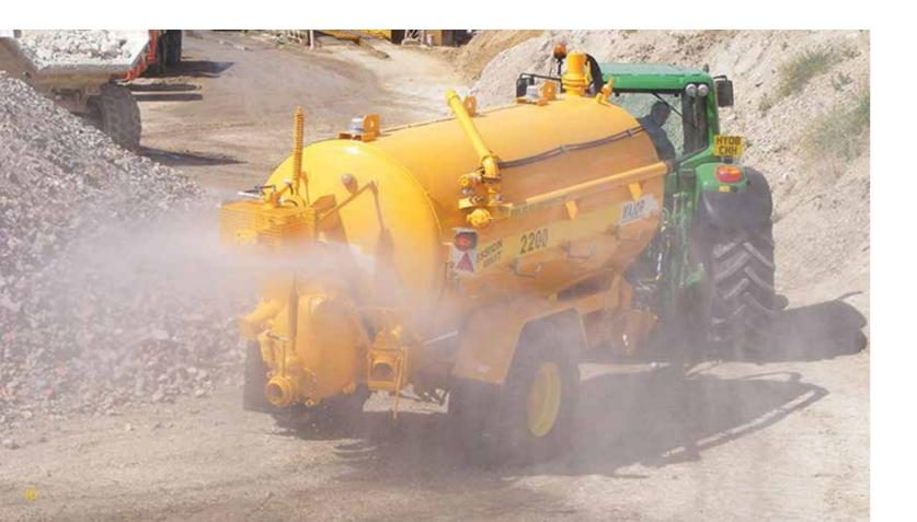
without compromising dust control levels. It eliminates flooding caused by traditional splash plate systems. This unit has significantly reduced Pinden's
