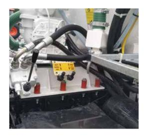
The pump exhausts through a muffler box for reduced noise and odour. An uprated hydraulic pump and PTO system were fitted to the truck in order to deliver the required hydraulic power. The 1,800 litre/400 gallon freshwater tank is filled from a fire hydrant instantaneous coupling but also has a standard garden hose fitting for use in emergency. Water levels can be monitored using a full length sight tube attached. A separate Lombardini 26hp diesel power-washer is mounted at the rear
