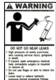
High oil pressure hazard
