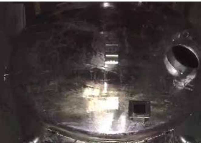
All Major tankers are galvanized inside and out for durability and long life.
