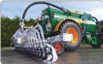
MAJOR 2050LGP with a 6.4m trailing shoe injector
