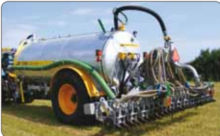
MAJOR 3100LGP with a 5.2m disc injector
