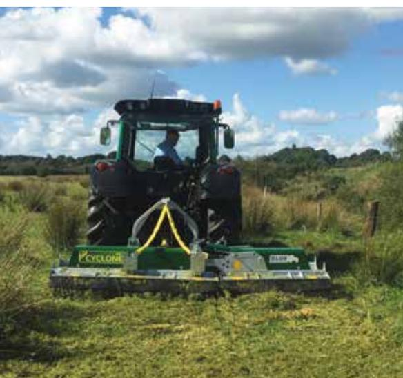
The award winning range of Cyclone Mowers has been designed to do the work of a flail mower but requires a fraction of the power and fuel that a flail mower would consume.
